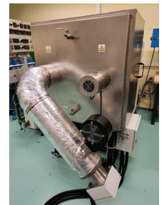
A prototype rotational molding machine built for the project
