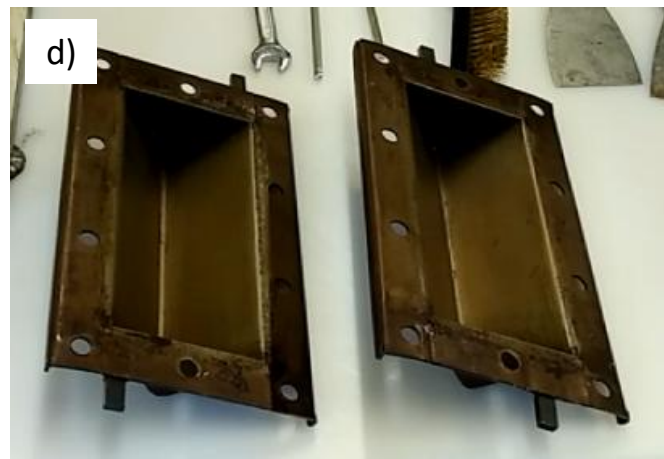
REMO GRAF single-arm shuttle rotational molding machine (a), products made of HDPE and HDPE-BC composite (b,c), steel mold (d).
